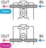
When used with two tubes and the assistance of a Y-pipe, it can function as a 3-way valve to divert fluids.
