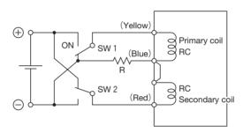
In either case, in order to cancel out the holding power of the permanent magnet on both coils (not just on the holding side), it is necessary to insert an external resistor (R) for degaussing. Thus, the unit operates on a two-loop structure.
