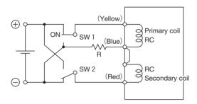
When switch SW 2 is turned on (with SW 1 off), the shaft is pulled to the secondary coil side. Even if switch SW 2 is reset the shaft maintains its position.
