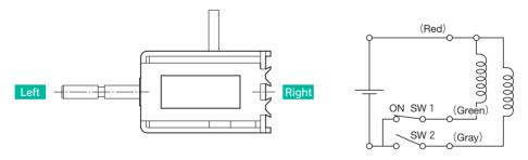
When switch SW 2 is turned on (with SW 1 off), the switch is pulled from left to right.
